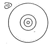
The Field should get weaker as you get farther from the wire, which means the lines should be farther agart as you go farther out.
