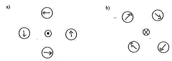
5. Each empty circle represents a conductor surrounded by a magnetic field. State whether a dot of an "X" should be placed in each circle.
